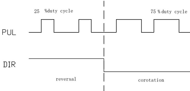
1. this control mode through the pulse duty cycle to control the speed, the effective duty cycle speed range is 10% ~ 90%, the corresponding speed range is 0 ~ (P06-40 setpoint) \*10. The recommended pulse frequency range is 1K ~ 20K. The corresponding formula between duty cycle and target speed is as follows:
