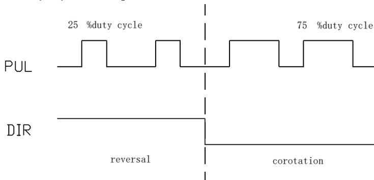
1.this control mode through the pulse duty cycle to control the torque, the effective duty cycle torque range is 10% ~ 90%, the corresponding torque range is 0 ~ (P06-43 setpoint) \*10. The recommended pulse frequency range is 1K ~ 20K. The corresponding formula between duty cycle and target torque is as follows:
